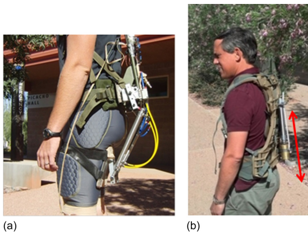
Fig. 9 (a) A powered exoskeleton is used to assist the torque needed at the hips [2]. (b) A powered PogoSuit is used to assist the hopping motion. A pneumatic cylinder oscillates the small mass up and down in phase with the user [4].
